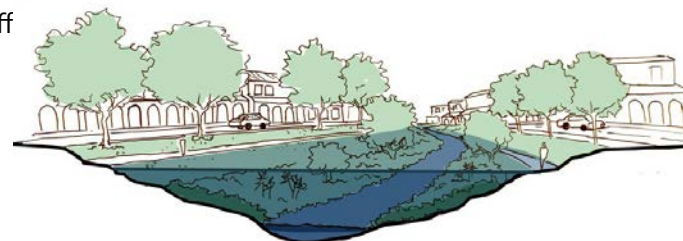
The sketches above show how public space can also serve to help with flood control. Most of the time, the space is green with a low flow channel and can accommodate trails and wildlife habitat. In the event of a large storm, the channel is designed to fill and provide expanded flood storage. The naturalized channel provides for beautiful long views and welcomes people to enjoy the space with trails and nature walks.
